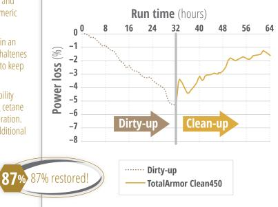
32 hour dirty-up (DU) with 1 ppm zinc in fuel 32 hour clean-up (CU) with 1 ppm zinc in fuel + additive
